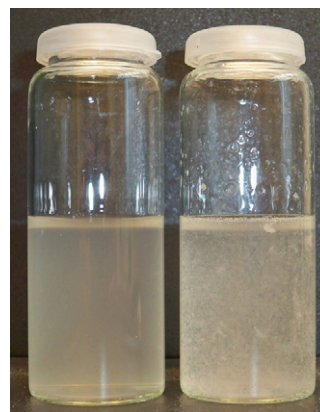
Fig. 3. Native XG (left vial) and PLLA-grafted XG (right vial) in water, after stirring and heating at 60 °C for 2 h.
